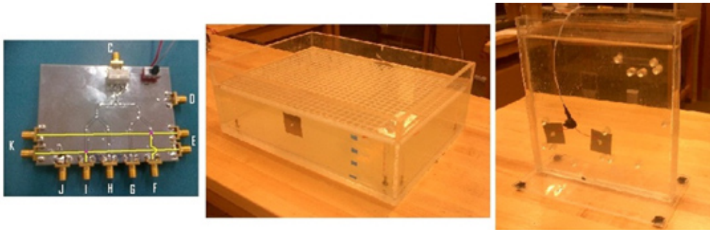
Figure 6: Tissue simulation devices: from left to right - tissue interface circuit, horizontal saline tank phantom, vertical saline tank phantom.
